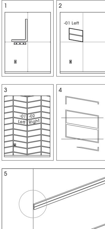
**Note:** Install panels on a flat, vertical surface only. Acclimate panels to room temperature for 24 hours. Construction adhesive installation is permanent and will cause surface damage if removed.
